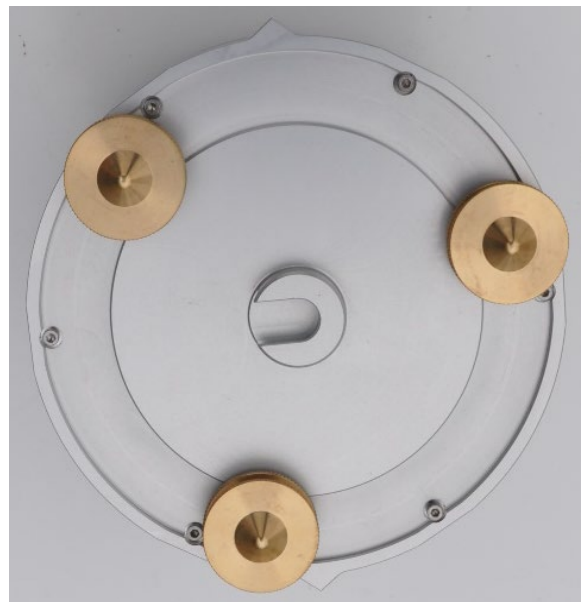
Figure 2 Accelerometer base with fixing point and Orientation indicators machined to the base of the sensor
