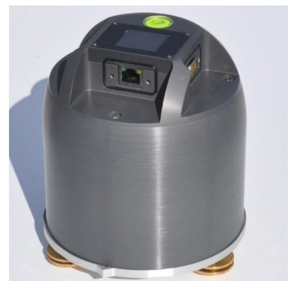
Figure 4 Feedback accelerometer with Encardio-rite D Type waterproof connectors
