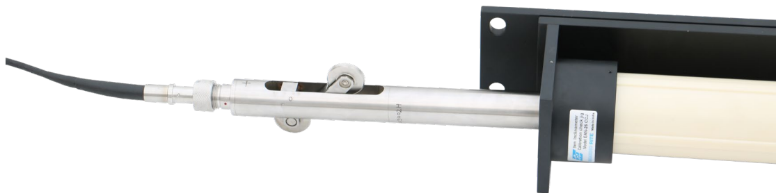
Figure 19 Calibration jig & inclinometer probe
