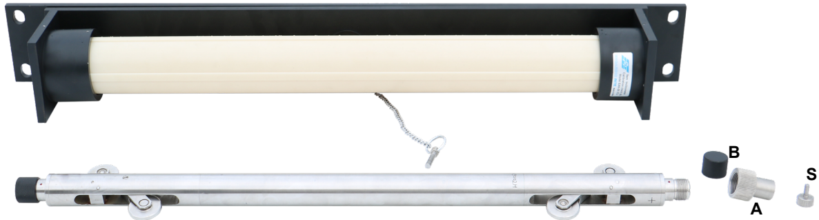
Figure 18 – Calibration jig & inclinometer probe with protective end cap, retainer cap and anchoring screw
