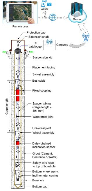
EAN-56 In-place inclinometer system with RF datalogger and gateway
