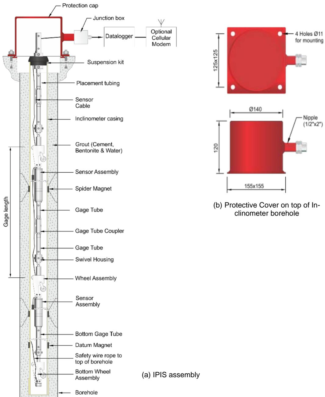
**Figure 3-1: In-place 3D Incliner cum Settlement assembly and Protective cover**
