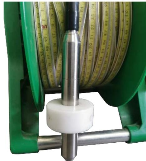
**Figure 4-5** Magnetic Probe with nylon disc
