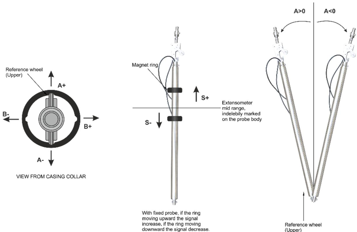
Figure 6-3 Displacement and Settlement Direction
