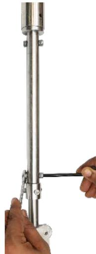
(c) Fixing sensor to gage coupler tubing
