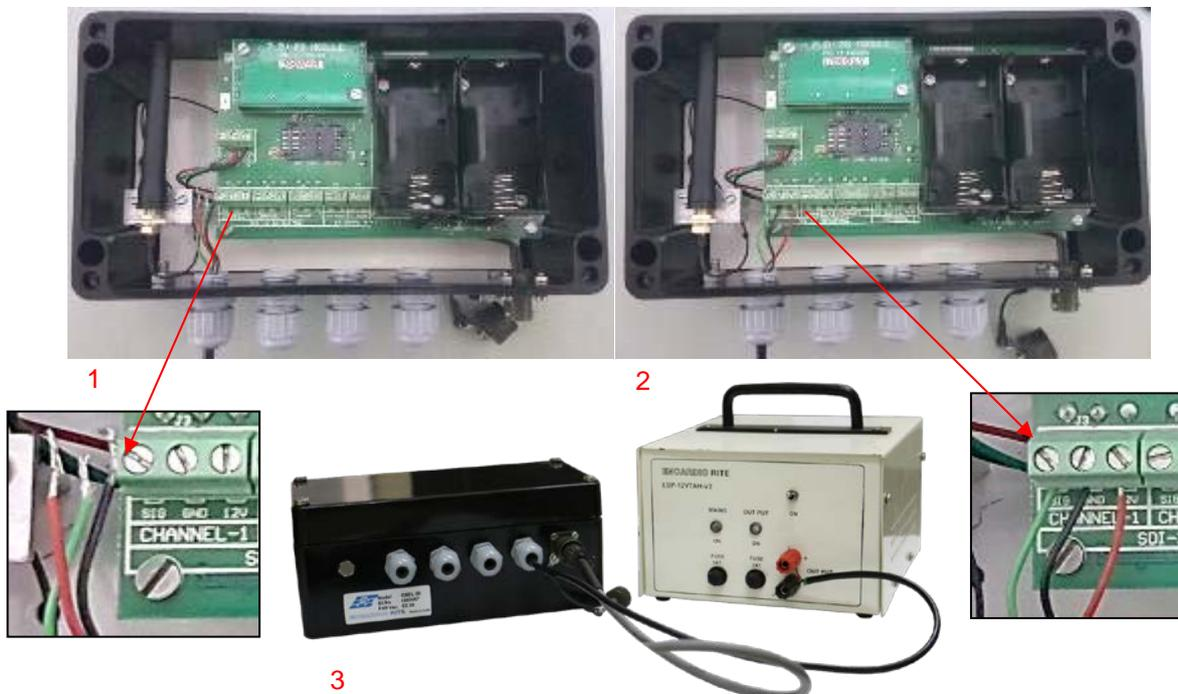
**Figure 7-1 Connection of IPIS with ESDL-30 Datalogger:**
