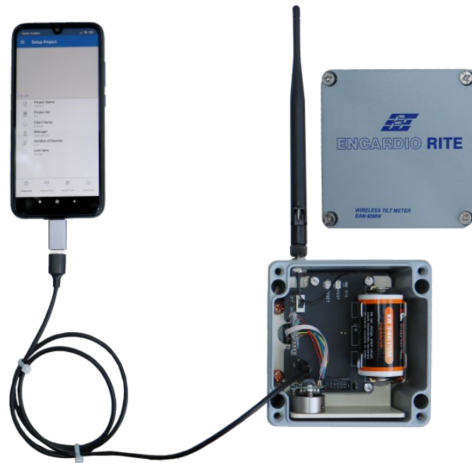
Figure 6-2 Tilt meter connected to Android phone with USB cable via OTG adaptor
