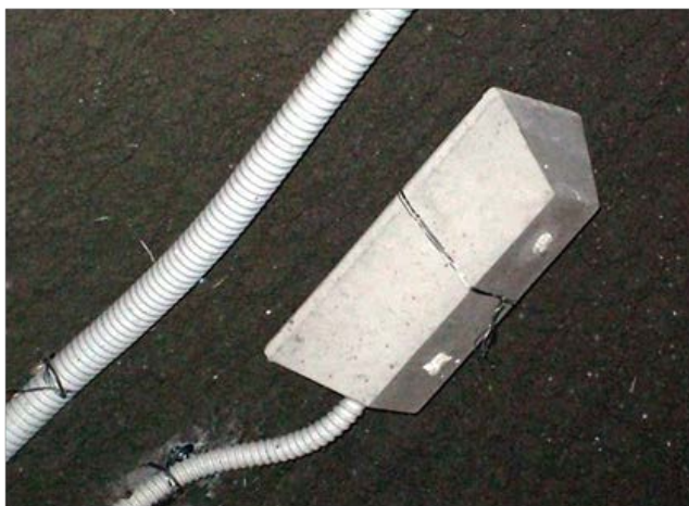
Figure 3.4 Strain gage casted in small concrete blocks for embedment in mass concrete
