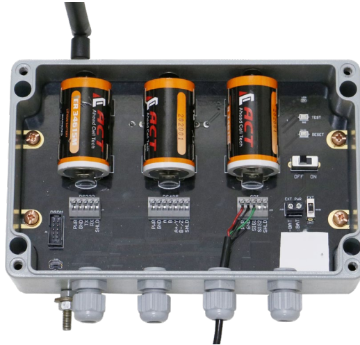
Figure 10-2 Connection of digital sensor with SDI-12 output to digital node
