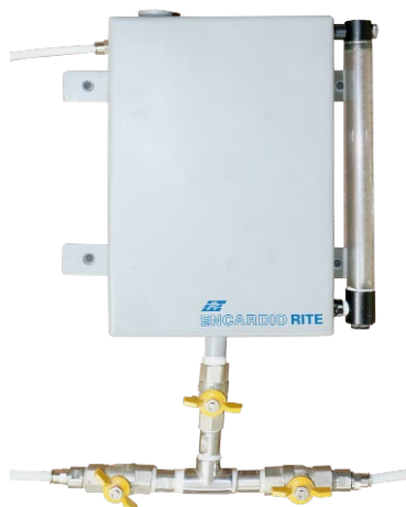
Figure 2-3 Reservoir (reference tank)
