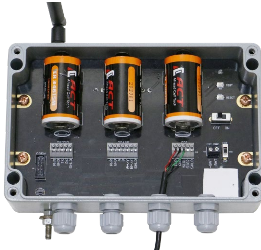
Figure 9-2 Connection of digital sensor with SDI-12 output to digital node
