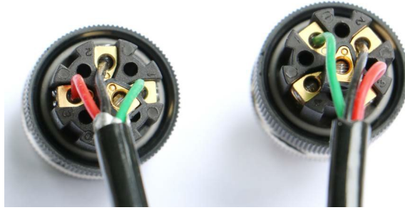
Figure 5-2 Wiring details for sensor with SDI-12 output
