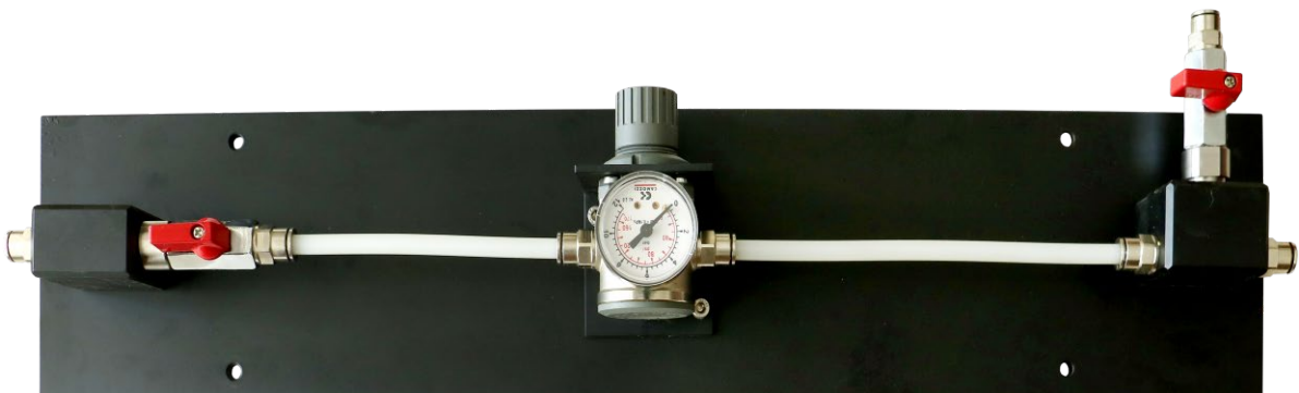
Figure 2-5 Gage and valve assembly
