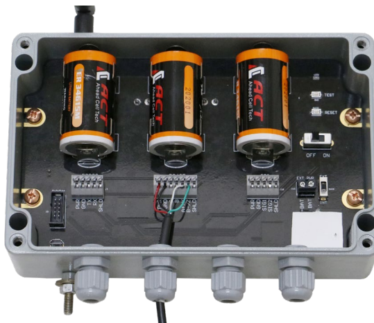
Figure 9-3 Connection of digital sensor with Modbus (RS-485) output to digital node
