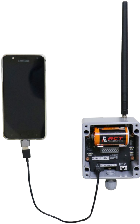
Android phone connected to single channel wireless node
